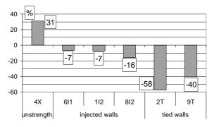
Figure 13: Transversal strain variation at the peak strength after injection and tying
