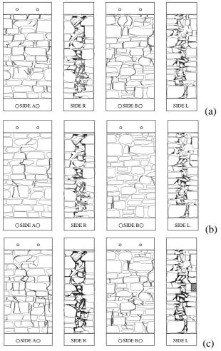
Figure 12: Cracks patterns at the same stress level before (a) and after (b) injection and after injection at the peak strenght (c)
