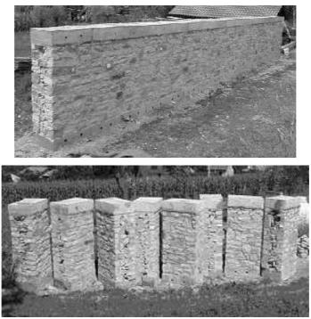
Figure 1 : View of the entire wall built and of some of the 17 specimens obtained after the wire sawing.
