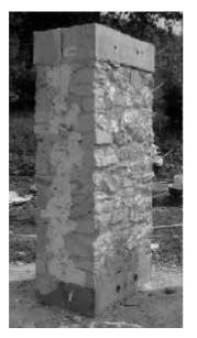
Figure 4: View of a wall before injection
